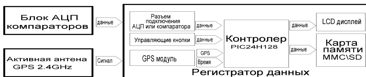
Fig. 1. Block diagram of data logger
